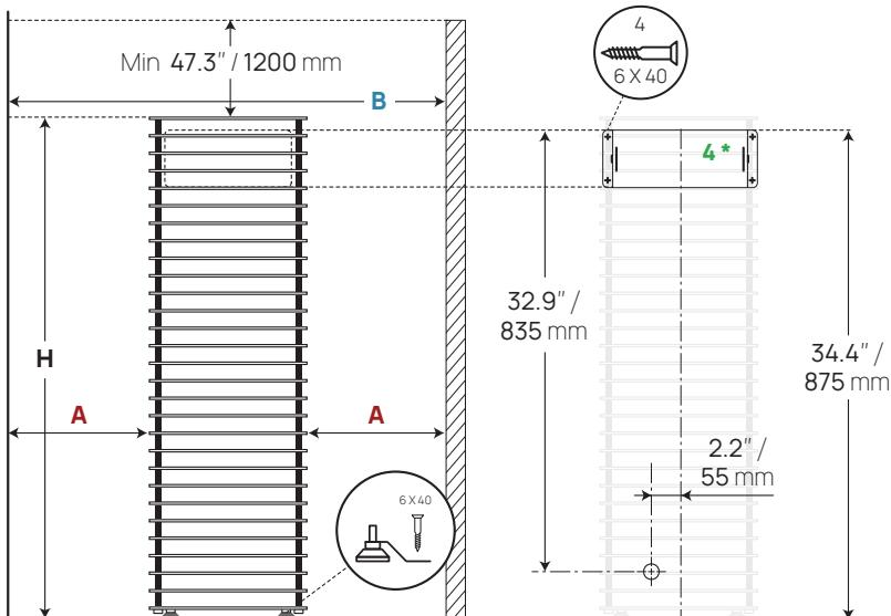
\* CLIFF Mini 4 is attached to the wall with a special bracket
