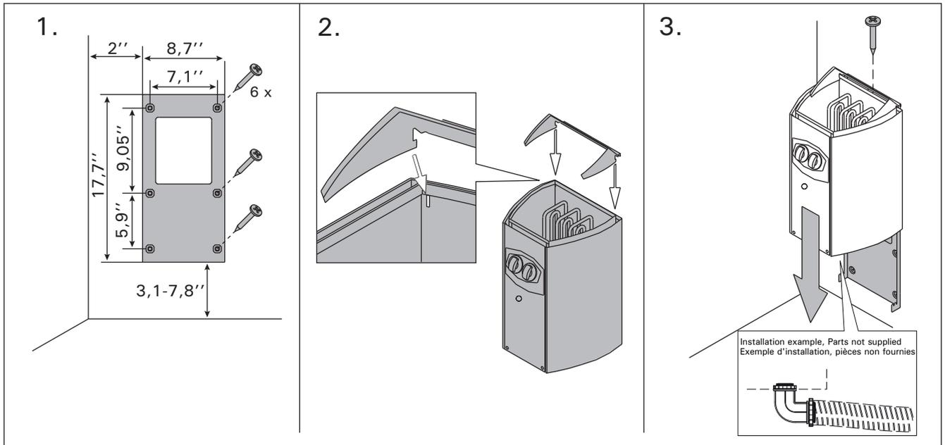
Figure 7. Installing the wall-mounting device (1.) and the heater (2.-3.)
