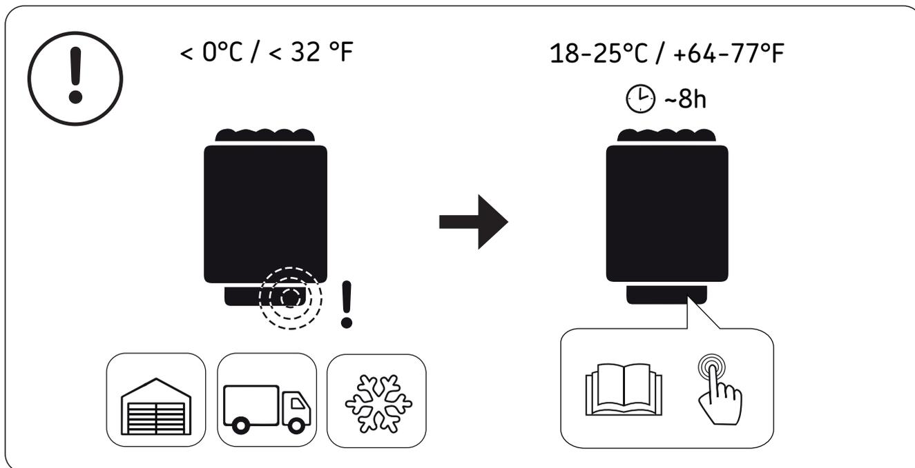
**!** Overheat protector of the device can go off also at temperatures below  $-5^{\circ}\text{C}$  /  $23^{\circ}\text{F}$  (storage, transport, environment). Before installation take the device to the warm environment. The overheat protector can be reset when the temperature of the device is approx  $18^{\circ}\text{C}$  /  $64^{\circ}\text{F}$ . The overheat protector must be reset before using the device. See the user manual > Resetting the Overheat Protector.
